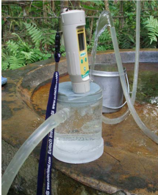
Figure 6. Flow through cell in which pH, EC and Eh-readings were taken.
